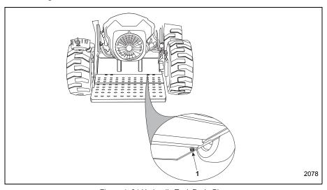
Figure 4-24 Hydraulic Tank Drain Plug
